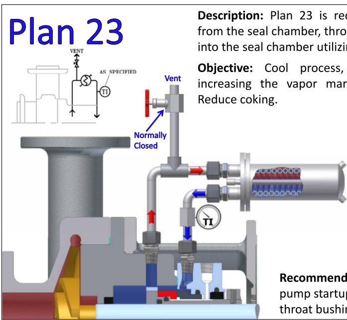
**Description:** Plan 23 is recirculation of process fluid from the seal chamber, through a seal flush cooler, back into the seal chamber utilizing a pumping ring.
